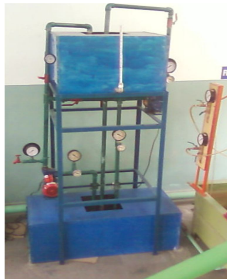
Figure. 4 Actual fabricated the centrifugal pump test rig
